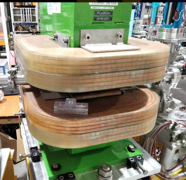
The active bending plasma device compared with a conventional bending magnet (Credit: INFN-LNF)
